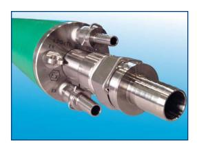
Each I-Fit connector consists of a hose barb fitting for connection to the tubing, O-rings for leak-proof sealing, threaded body for connection to the pump, and securing clip to hold the pieces together.
